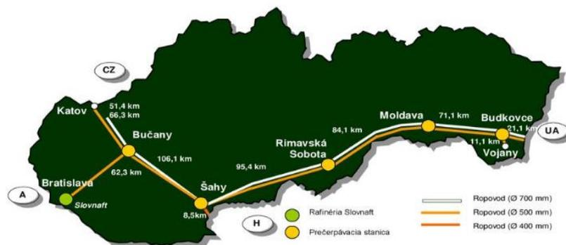
The length of the pipeline on Slovakia’s territory between the Ukrainian and Czech borders is approximately 444 km and includes five pumping stations (PS1 Budkovce, PS2 Moldava nad Bodvou, PS3 Rimavská Sobota, PS4 Šahy-Tupá, PS5 Bučany). The Druzhba pipeline as well as other minor crude oil pipelines in Slovakia are solely in possession of TRANSPETROL, a.s., a 100% state-owned company
